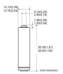
Chemical System: Alkaline Zinc-Manganese Dioxide (Zn/MnO<sub>2</sub>)
